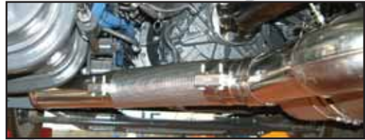
Fig 16 – typical flex pipe installation
