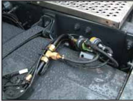
Fig 3. Typical Injection point assembly arrangement
